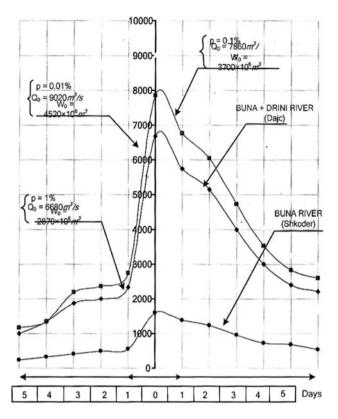
Fig. 74.2 Maximal flow, Buna + Drini River-Dajg
