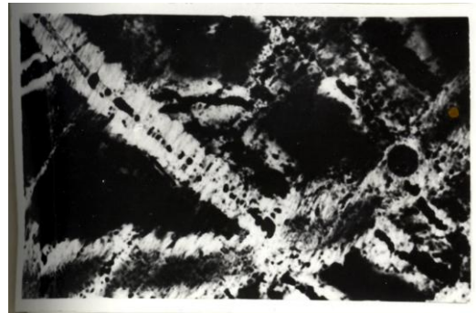
Photo 1. Serpentinite from dunite, with fissures of different ages, chrysotile-asbestos and magnetite, Kam deposits. Magnetic susceptibility \chi > 3000 \cdot 10^{-5} units SI. Thin section, enlargement 35x, Nicoles parallel. (Frashëri A. et al. 2008).
