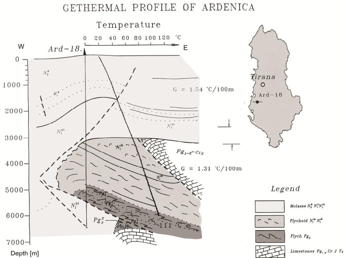
Fig. 8. Geothermal profile, Ardenica Molasse struture
