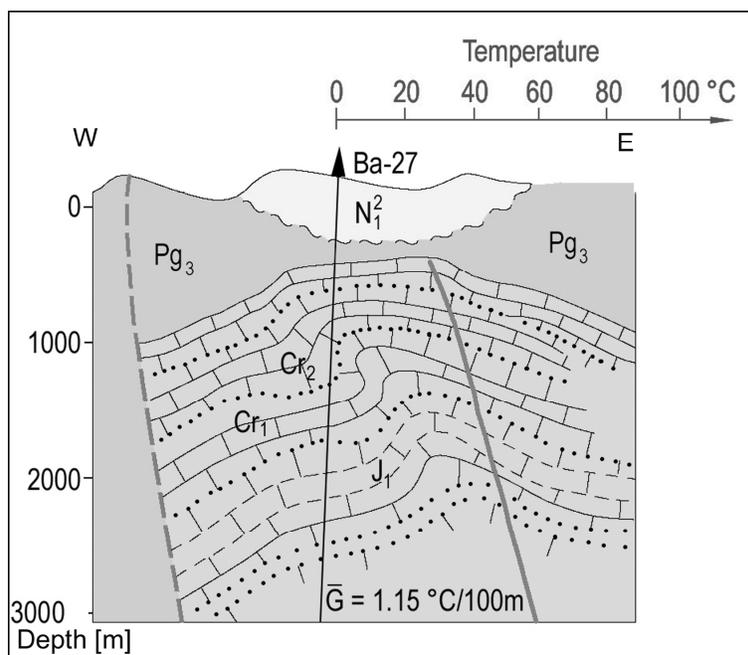
Fig. 6. Geothermal profile, Ballshi carbonate structure.
