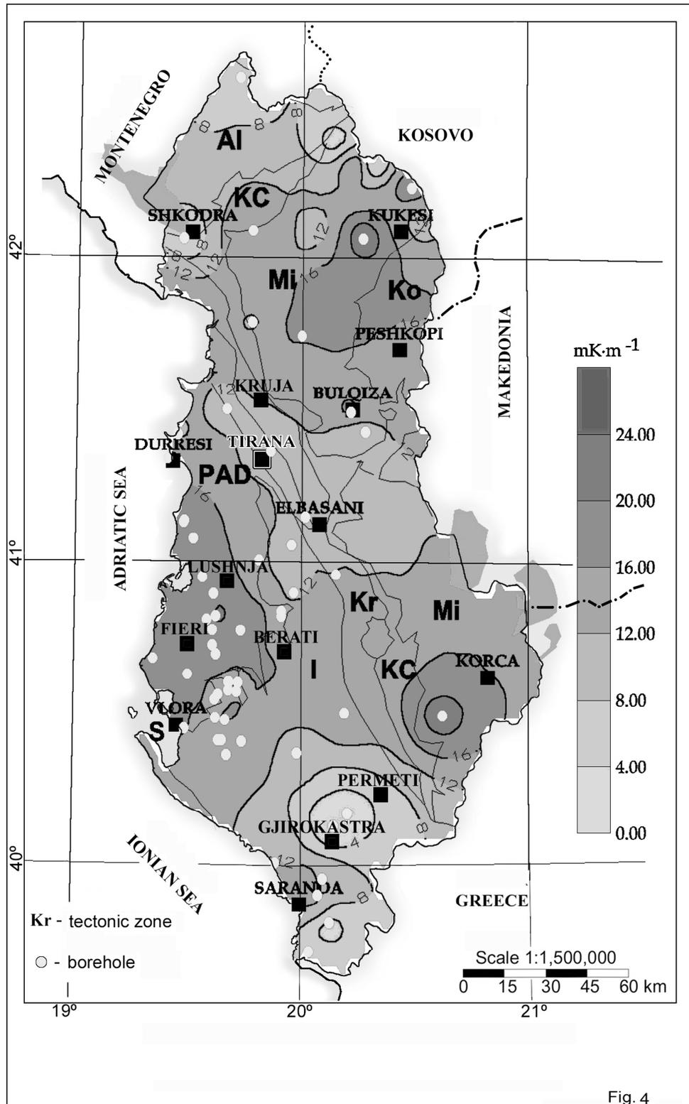
Fig. 4. Average geothermal gradient map of Albania.
