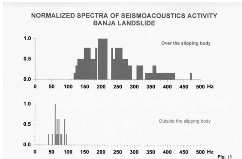
Fig. 2.10. Normalized spectra of seismoacoustic activity, Banja Landslide
